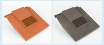
A neat and compact design that will maintain the aesthetics of a plain tile roof. This vent is designed for use with the standard 265mm x 165mm plain tile, replacing only 3 tiles without the need to cut any roof battens or surrounding tiles.
